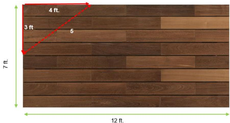
If the third measurement is 5, you know the corner is square. If it is not 5, ensure the measurements of the two sides are 3 and 4.
